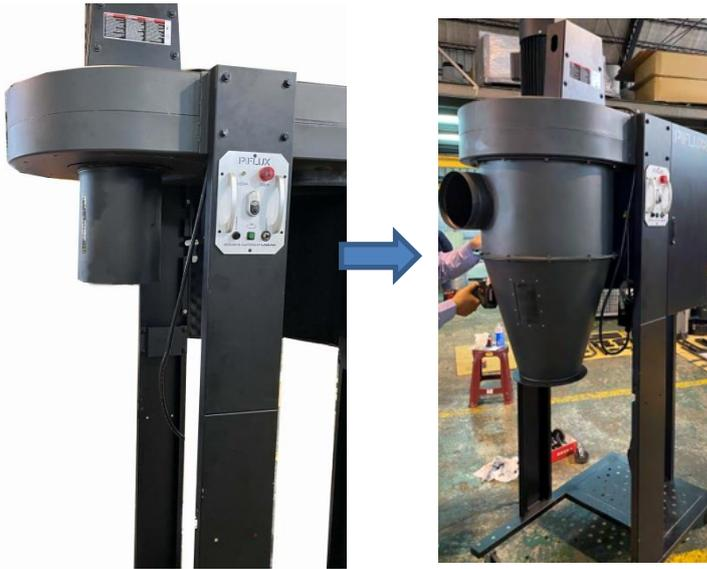
8. Attach the intake cylinder to the dust chute using (4) 5/16"x5/8" hex spring bolts. Then, attach the cyclone barrel onto the dust chute using (12) 5/16"x3/4" hex bolts and (12) 5/16"x18x2mm flat washers followed by attaching the cyclone funnel to the barrel using (12) 5/16"x3/4" hex bolts, (24) 5/16"x18x2mm flat washers and (12) 5/16" hex nuts.
