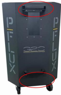
31. Attach the handles to the top and bottom end on the front panel with the window display using (4) flat head Philip bolt, (4) 5/16" x 7/8" flat washers and (4) 5/16" hex nuts. Note that the head of the Philips bolt must be inserted from the handle with the hex nut and washer on the inside of the drum.
