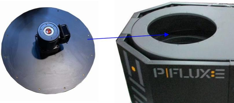
10. Attach the auto clean plate to the dust chute using (12) 3/16"x1/2" sheet metal bolts
