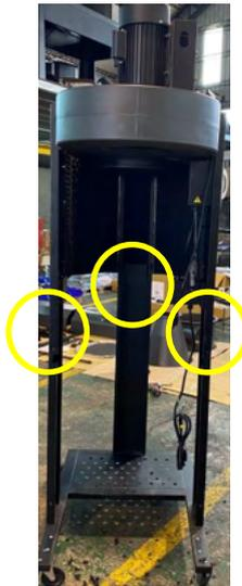
6. Secure the (3) upright support reinforcement plates using (12) 5/16" x 3/4" hex bolts and (12) 5/16" x 1" flat washers.
