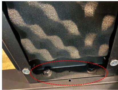
2. Remove the base which has been bolted to the (3) top upright supports. Keep the (6) 3/8"x3/4" hex bolts and (6) 3/8" flat washers for assembling the lower supports to the base. Keep the upper assembly lifted for step 5.
