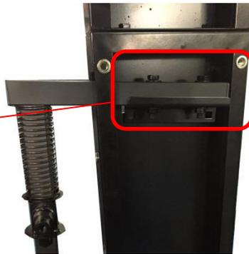
19. Secure the top end of the foot pedal bar to support bracket using (4) 5/16"x1-3/4" hex bolts, (8) 5/16"x18x2mm flat washers and (4) 5/16" hex nuts. Make sure the foot pedal bar is pushed all the way to the end of the support bracket (indicated by yellow arrows). Follow the same steps for the opposite side.
