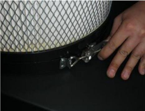
**Figure 8: Releasing filter clamp**
