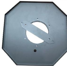
29. Attach the crossbar to the drum lid and tighten using the two bolts removed in the previous step. It does not matter which position you attach the crossbar.
