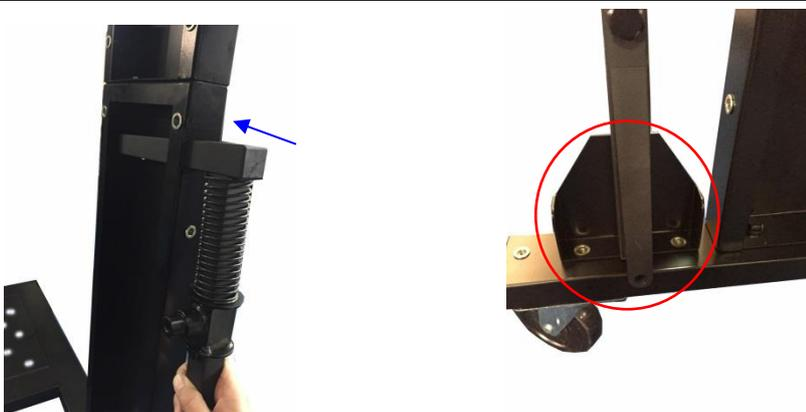
18. Ensure that the foot pedal bar is the correct side and slide the Foot pedal bar into the opening on the lower upright support panel. Make sure the end of the bar is on the inside of the triangular support plate. Follow the same steps for the opposite side.
