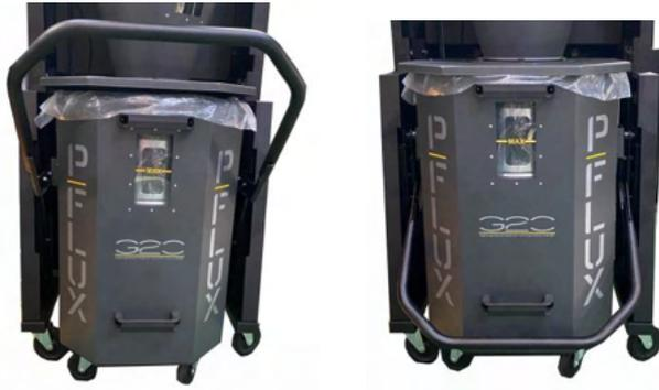
39. Lift the foot pedal bar. Align the Octagon drum window to the center point of the drum lid and push the drum in. Lower the foot pedal bar to seal the drum tight for normal machine operation.
