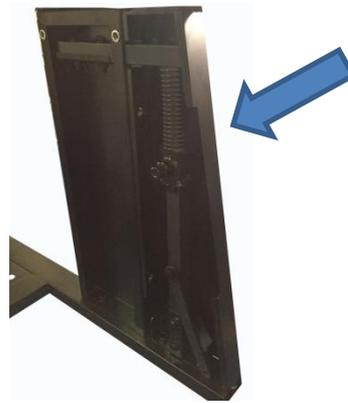
21. Attach the cover plate over the foot pedal assembly. Secure using (6) 1/4"x3/4" hex bolts and (6) 1/4"x19x2mm flat washers. Follow the same steps for the opposite side.
