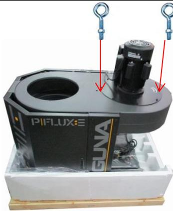
1. Remove (2) 5/16" x 5/8" hex bolts on the motor plate (shown by red arrow). Install (2) 5/16" eye bolts (not supplied) on the motor plate. With the help of another person, lift the upper cyclone assembly using a forklift. Make sure to hold the opposite side of the dust chute to prevent swaying while lifting the assembly up.
