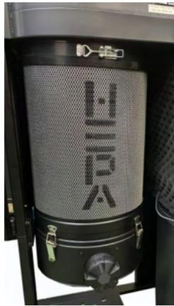
15. Attach the canister filter end cap to the canister filter using the (4) latches. Cover the 4" hook up with the 4" rubber plug.
