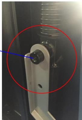
22. Attach the two ends of the Octagon foot pedal to the nut on the foot pedal bar.
