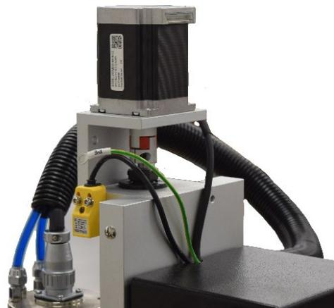
**Figure 2-5: Stepper Motor**
