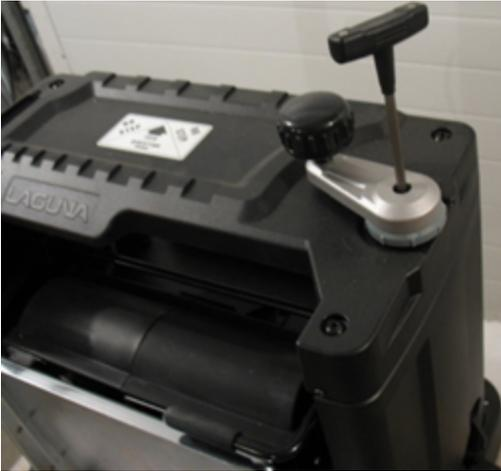
Figure 3: Thickness Adjustment Handle
