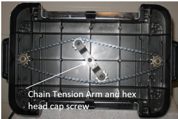
Figure 16: Under view of planer showing chain configuration.
