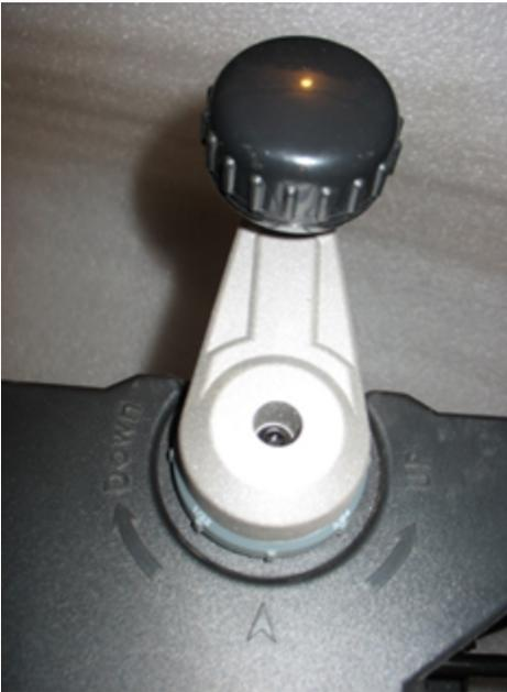
Figure 12: Thickness Adjustment Handle
