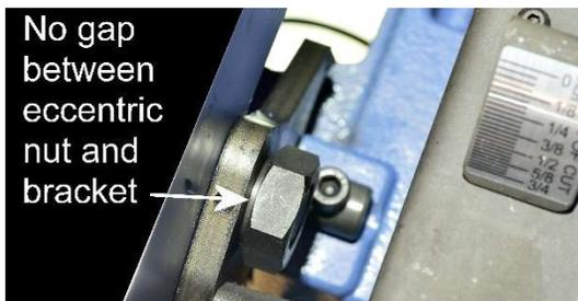
13. Adjust infeed / outfeed table parallelism using the infeed table eccentric nuts. Repeat the steps in "Inspect Outfeed Table Parallelism" when making adjustments. Again, leave no gaps between eccentric nut and the bracket.
