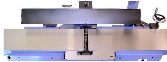
This fence comes with an auxiliary fence for jointing thin stock. When not in use, it can be securely hung on top of the main fence with the fence hanging notch.
