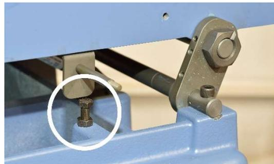
4. The stop nut for finishing passes is located below the infeed table, near the height adjustment worm gears. This stop nut should stop the table with 1/32" depth of cut. Loosen the jam nuts when making adjustments.
