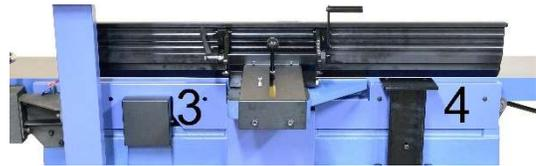
5. Each panel is secured by two cap screws, which are covered by plastic caps. Use a straight head screwdriver remove the plastic cover, then remove the hex cap screw with a 5mm hex wrench.
