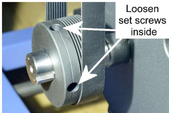
5. Realign the motor pulley with the cutterhead pulley.
