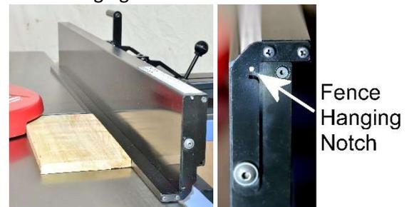
**IMPORTANT:** When deploying the auxiliary fence, please be sure the plastic supporting plates are sitting between the auxiliary fence and the table. Without these plates, the cutterhead will strike the auxiliary fence.
