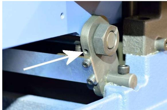
8. The eccentric nuts should be fairly loose once they are unlocked. Rotate the eccentric nuts to align outfeed table and cutterhead.
