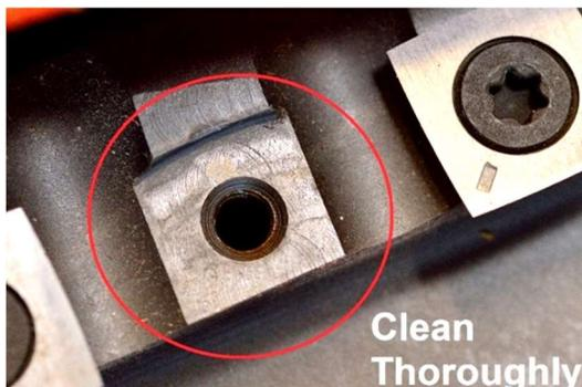
**IMPORTANT:** Obstacles between the insert and cutterhead platform will create uneven pressure against the insert. This will lower cut quality and may cause the insert to crack.
