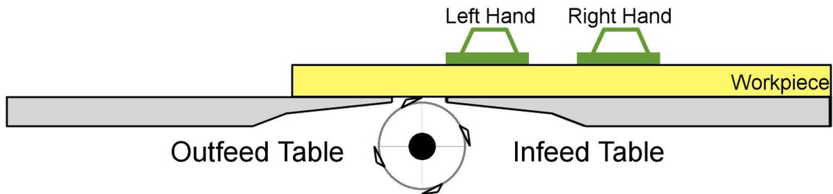
8. As left hand approaches the cutterhead, lift it up and move across the cutterhead to avoid accidental contact. Put left hand on stock that sits on the outfeed table, and continue to feed. Maintain control of stock with right hand while repositioning left hand.
