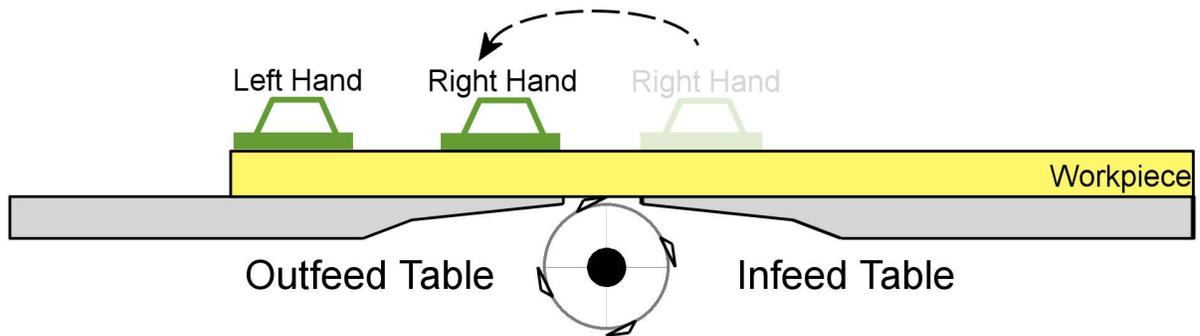
10. From this point on, continue feeding only on outfeed table until the entire length of stock has moved across the cutterhead. Maintain feed rate to produce smooth cut with no burnt marks.
