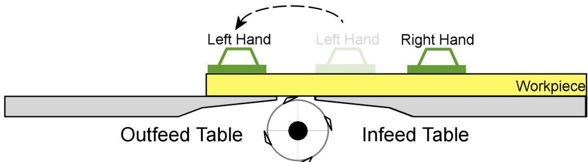
9. As the right hand approaches the cutterhead, reposition right hand as shown in the diagram. Operator should move forward and continue feeding next to the outfeed table. Maintain control of stock with left hand while repositioning right hand.
