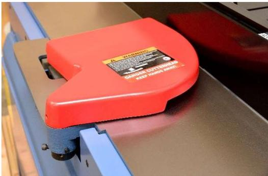
3. There is a spring-loaded knob at the bottom of the rabbeting table. It has a cap screw which grabs the cutterhead guard shaft and keeps the guard pushing against the fence.
