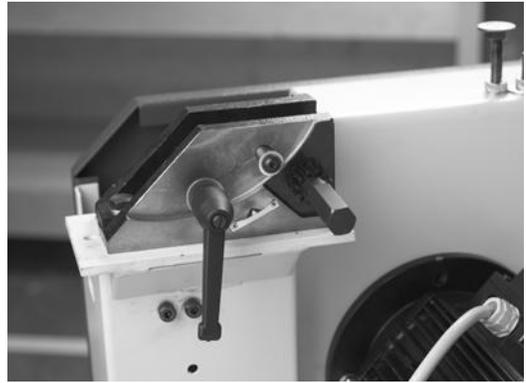
2. Position the table on the trunnion, taking care not to damage any of the table or trunnion surfaces.
