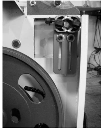
**Note:** Rotate the back guide by approximately 15 degrees after every 8 hours of use. This will greatly extend the life of the back blade guide, as it will even out the wear.
