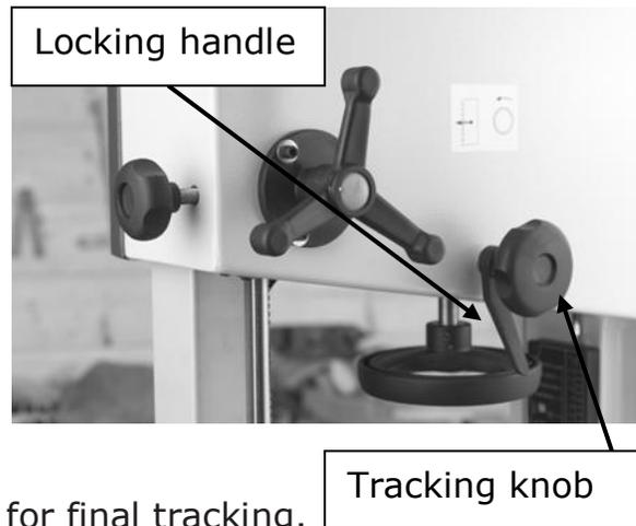
**Note:** The blade must be fully tensioned for final tracking.
