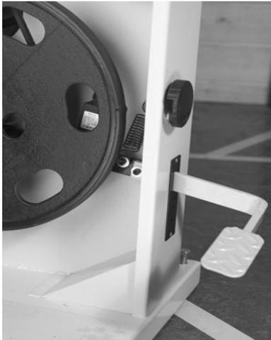
Should the blade break, this guard protects the operator from the blade escaping under the table. To assemble the guard remove the thumbscrew that you will find stored on the inside of the door.
