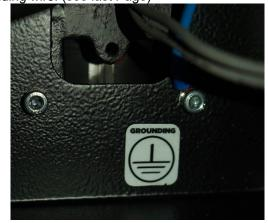
If repair or replacement of the electrical cord or plug is necessary, do not connect this equipments grounding wire to a live terminal. Check with qualified electrician or service personnel if the grounding instructions are not completely understood or in case of doubts whether the Dust Collector is properly grounded. Use only 3 phase extension cords that have 3 hot wires a ground wire. Confirm that the plug for your Dust Collector is compatible with the 3 phase receptacle it will plug into.
