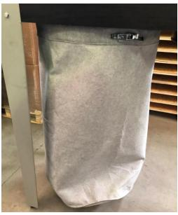
10. If you use drums, fasten the sleeves to the dust collector flange and place the drum underneath, then fasten the bottom of the sleeve to the steel drum. (**drum not included**).
