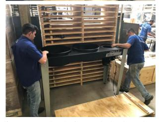
4. If necessary, adjust the feet attached under each leg:
