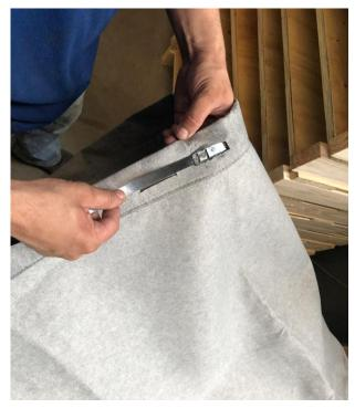
8. Slide the filter bag loop over the hanger hook (repeat this process twice):
