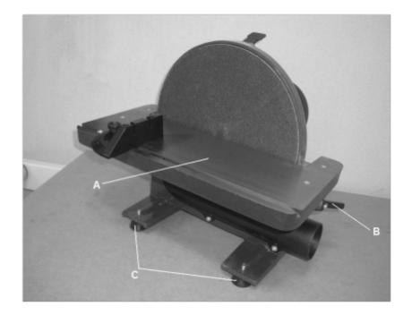
position on a smooth and level surface and check that the machine is stable, without oscillating. If necessary, turn again and adjust the feet so that it does not sway when in the correct position.
