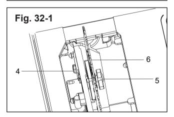
necessary to remove the blade guard and kickback pawl when using the dado.
