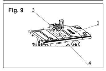
**WARNING:**Improper alignment of the splitter can cause "kickback" and serious injury.
