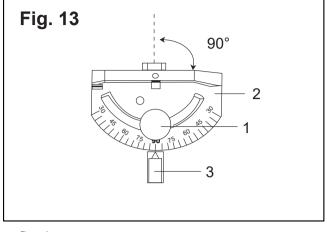
3. In order to change the angle of the mitre gauge, loosen the locking handle (1) and the rotate the mitre body to the desired angle, as indicated on the scale. Tighten the locking handle in order to hold the mitre body securely in position.
