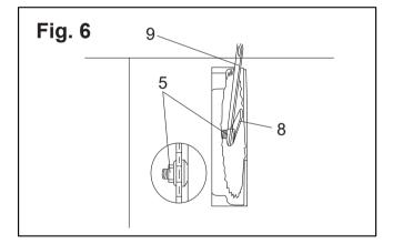
**WARNING:** VERIFY THAT THE SAW BLADE, THE ARBOR FLANGE, AND THE NUT ARE PROPERLY SEATED. AND THAT THE ARBOR NUT IS TIGHTENED SECURELY.
