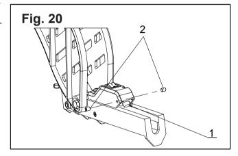
4. Using a hex wrench (not provided), adjust the laser unit (1) until the laser line is parallel with the blade.
