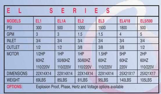
Hydrostatic Test Pumps () Post Hole Diggers
