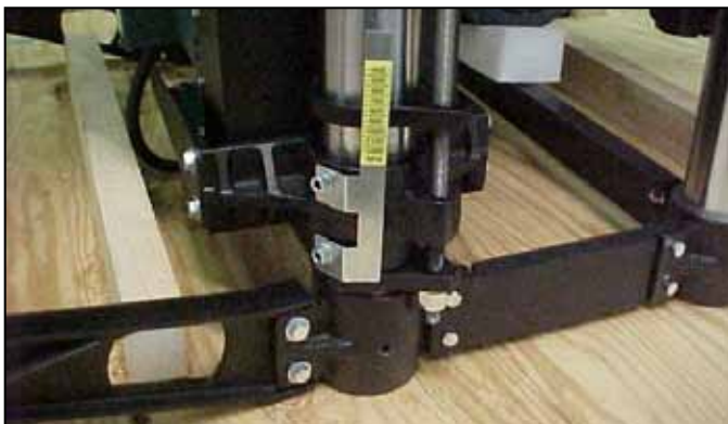
Fig. 8. Brush RPM gauge
