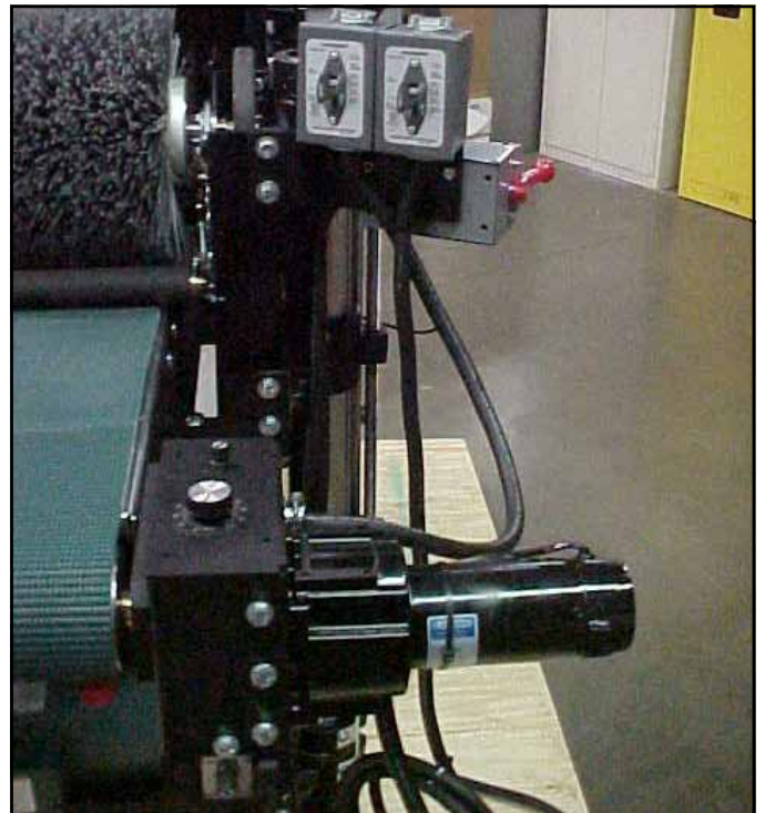
Fig. 26. Conveyor motor control box and brush on/off switches.
