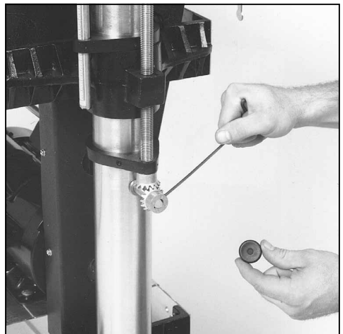
Fig. 14. Adjusting miter gears for proper mesh.
