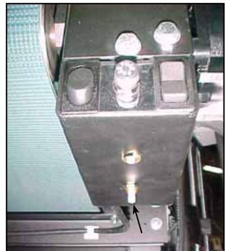
Fig. 10C. Variable speed control, height adjustment.
