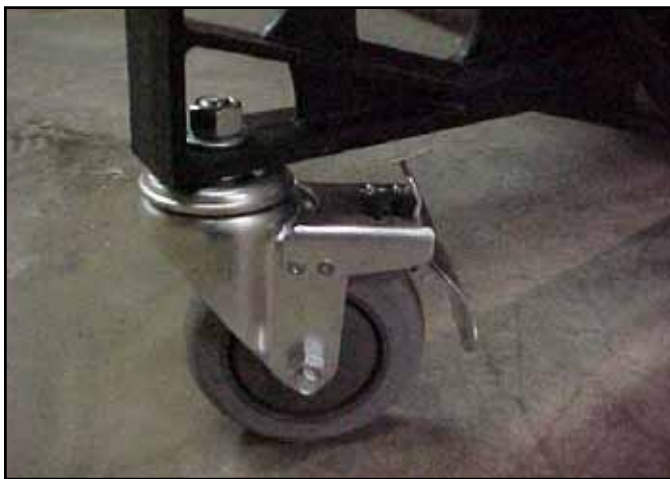
Fig. 2. Caster and mounting hardware.
