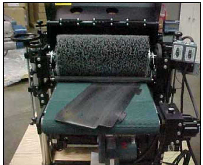
Fig. 12B. Offset stock feeding angle, metal.
