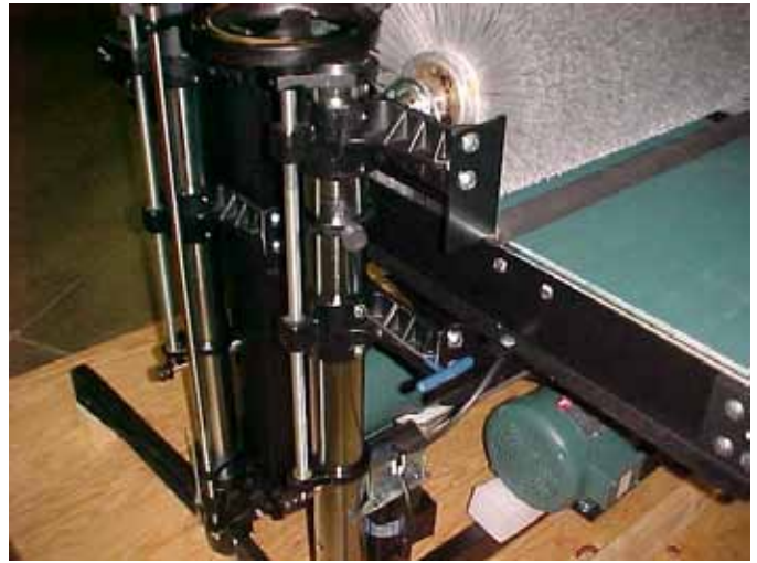
Fig. 6. Checking brush alignment and table height adjustment (outboard side).
