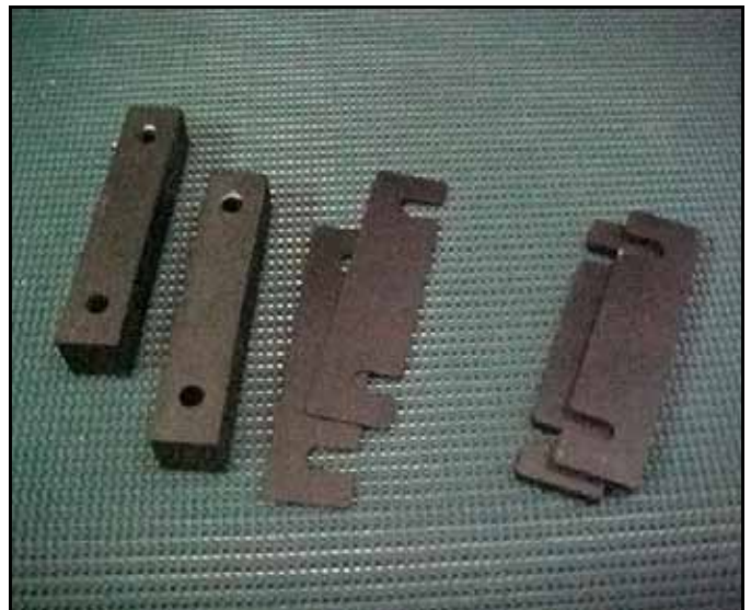
Fig. 12D. Shims. Rear brush contact adjustment.
