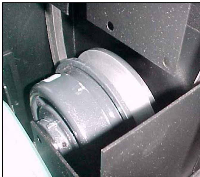
Fig. 24. Removing main motor V-belt.
