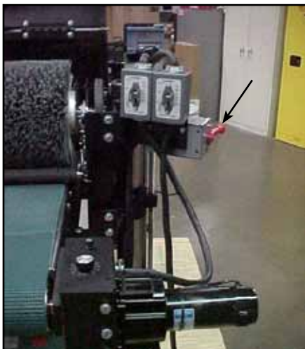
Fig. 10A. Forward/Reverse switch, Rear head.
