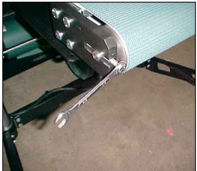
Fig. 21. Tensioning and tracking conveyor belt.
