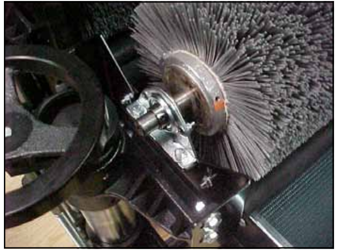
Fig. 19. Removing brush head.
