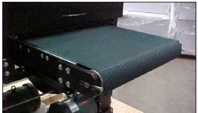
Fig. 9. Adjusting conveyor belt tracking.
