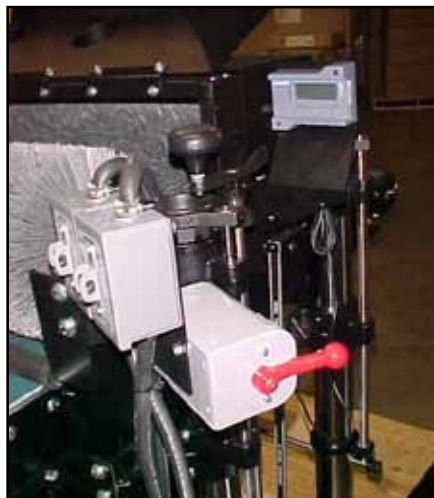
Fig. 10B. Forward/Reverse switch, Rear head.
