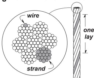
*Wire rope assembly must be replaced if more than 6 wires are broken in one lay, or if more than 3 wires are broken in one strand in one lay.*
