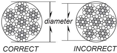
The wire rope assembly must be replaced if the diameter measures less than the minimum diameter at any point.
