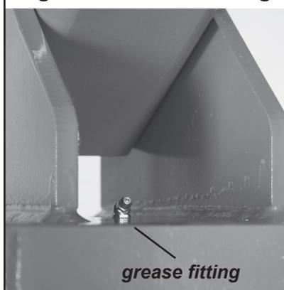
Figure 5 – Mast Rollers
