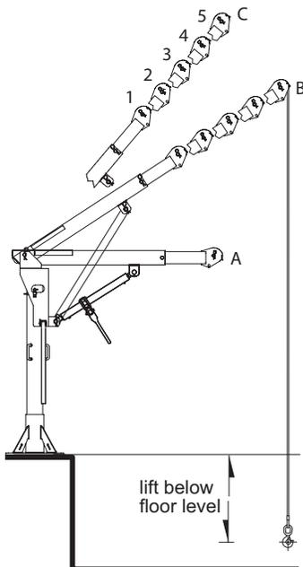
Positions A and C require models equipped with ratchet jack.
