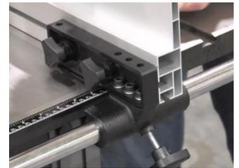
NOTE: If fence needs to be adjusted, nylon slider nut on the inside of the casting to adjust fence up or down. There are also 2 set screws on the side of the casting that adjust the angle of the fence.
