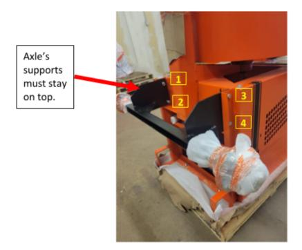
4.- Remove all the nuts (8) from both axle's hubs. Mount the wheels on the hubs making sure the air valve is facing outside. Tighten the the 8 nuts at no more tan 105 ft/lbs.
