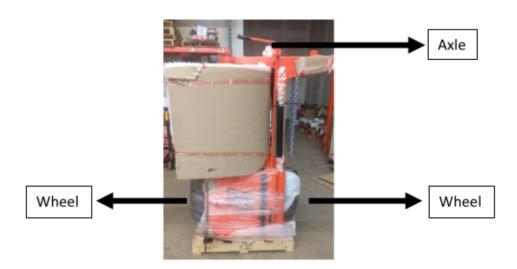
2.- Unpack: cut straps, remove all cardboard, plastic wrap and packing material from the unit. Remove the axle and wheels from the mixer. Remove the bolts (4x %" x 1-3/4") and nuts (4x %") that come attached to the axle's supports.
