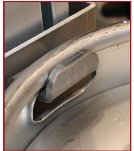
Lifting bracket holds kegs securely in place during transport and lifting
