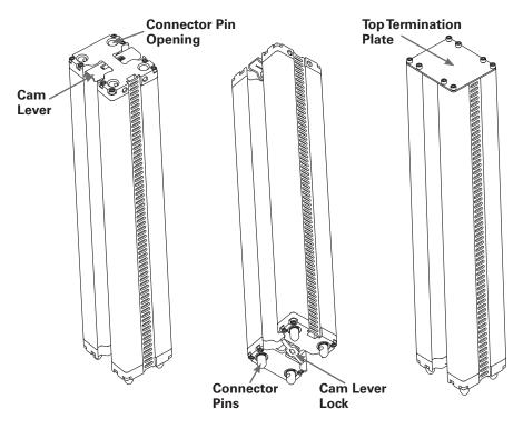
Figure 2-7 - Mast Connectors
