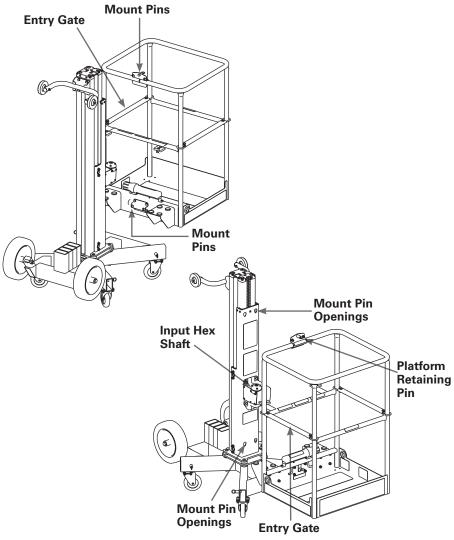
Figure 2-6 - Platform Mounting and Retaining Pins
