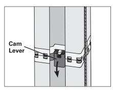
**3.** Press both cam levers down and in at the same time.
