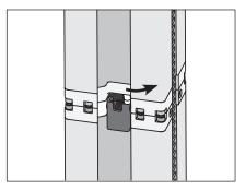
**4.** With the cam lever in the down position, be sure the cam lever lock springs automatically into the locked position.
