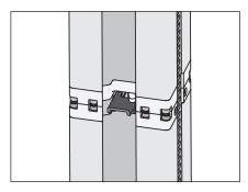
**1.** Stack the mast ensuring that the track is facing toward the platform.
