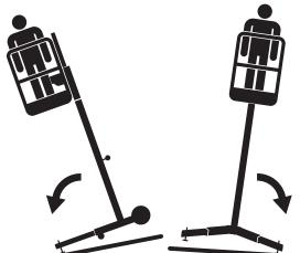
• Check to be sure the chassis is level according to the bubble level indicator on the chassis and all wheels are completely off the ground. Note: the platform will not release from its docked position unless each outrigger is in its proper position, fully extended and bearing weight.
