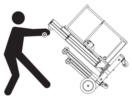
Figure 3-8 Maneuvering when tilted back
