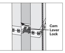
**2.** Rotate the cam lever lock until it stops in the center position.
