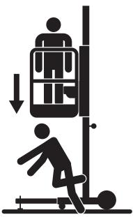
Warn personnel not to work, stand or walk under an elevated platform. Position barricades on the floor as necessary.
