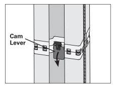
**1.** Press both cam levers inward to allow the cam lever lock to rotate freely.
