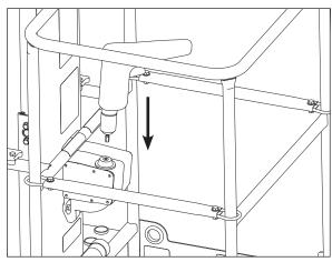
Figure 3-5 Drill Motor Operation / Elevating
