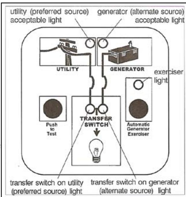
2. Turn on the preferred source (utility) circuit breaker. The utility source acceptable light should now come on as well as the transfer switch on utility light. If these lights fail to come on recheck your incoming power to insure you have 240 volts nominal. If not, troubleshoot your utility source before continuing.
