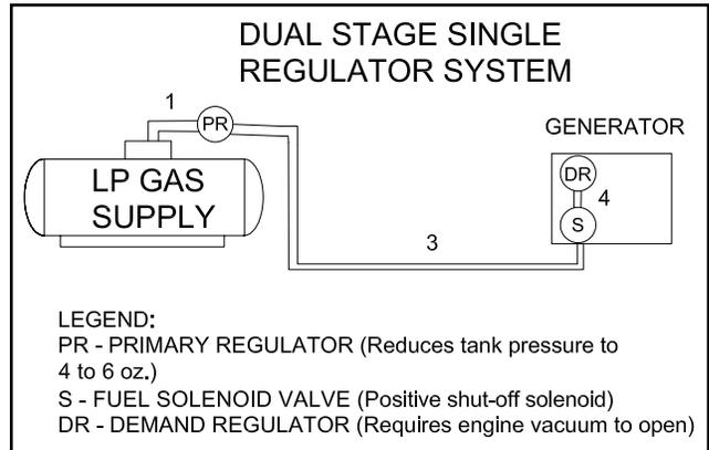
Reference numbers 1 through 3 in the diagrams above are system parts supplied by the customer.
