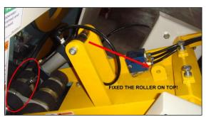
Make sure to lift up the front roller and fix on top when saw blade is higher than 60mm, nor the roller will be cut by blade!
