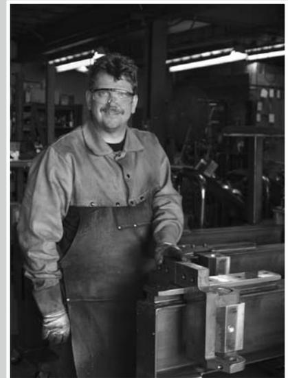
Mark Jeffords with the welded heavy-duty I-beam frame for a Huth bender.
