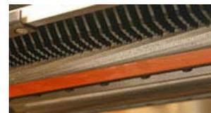
The all-metal adjustable feed rollers, anti-kickback fingers and adjustable chip breaker make this an exceptionally safe and user-friendly planer.
