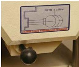
Dual feed rates allow quick dimensioning of the wood and then slowing the material speed for highly refined finish cuts.
