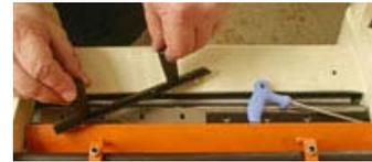
Our Quick-change knife system makes this once frustrating task quick, simple and automatically accurate. We include a pair of magnetic tools - shown here removing a knife retainer plate - that helps prevent nicked fingers!
