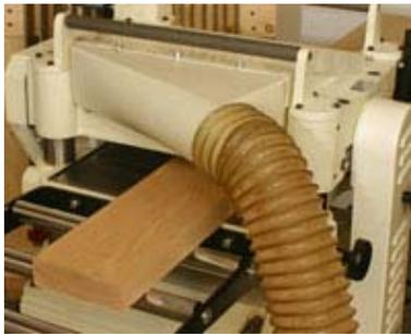
The 4"-diameter dust port is angled to the side to prevent the dust collector hose from interfering with the wood as it exits the planer.
