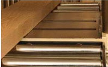
Adjustable height rollers in the primary table (left) make moving rough stock through the machine easier. The large roller extension tables (right) increase the overall table support to 48" long!
