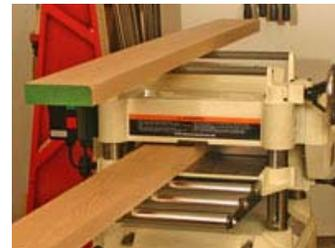
The heavy duty material rollers on top make returning heavy stock for the next cut easier and safer.
