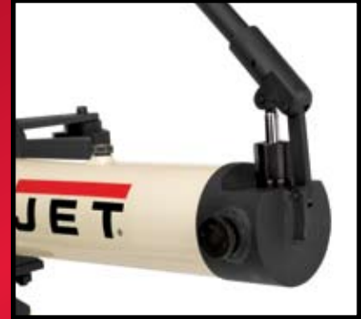
Heavy-duty hydraulic cylinder capable of bending schedule 40 pipe
