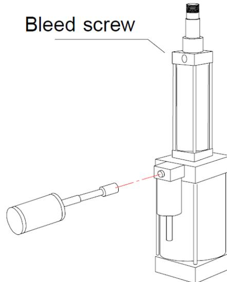
1. Put the head in the upper position in the mechanical stop.
