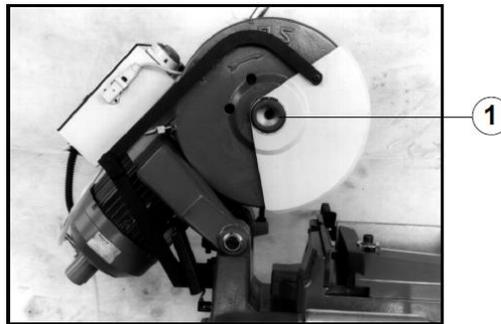
1. Release the blade guard and push it back as far as it allows.
