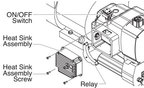
4. Disconnect the switch wires from the sprayer ON/OFF switch. Remember the locations of each of the two wires (label the wires, if necessary).
