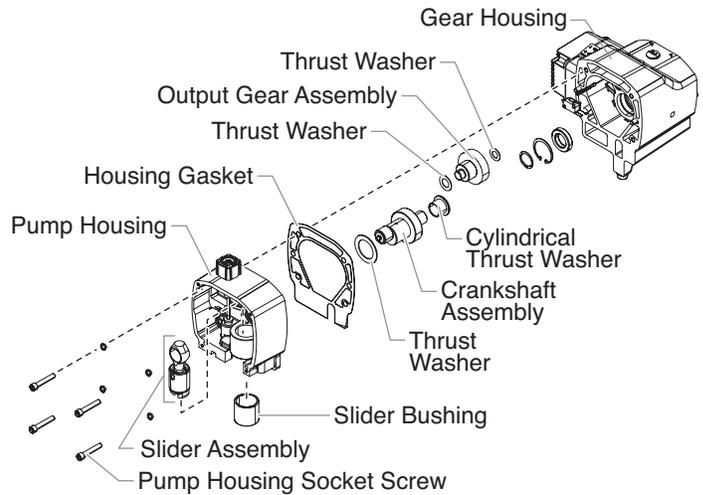
9. Slide the pump housing away from the gear housing.
