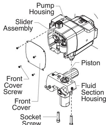
7. Slide the fluid section housing and piston rod forward until the piston rod is out of the T-slot on the slider assembly.
