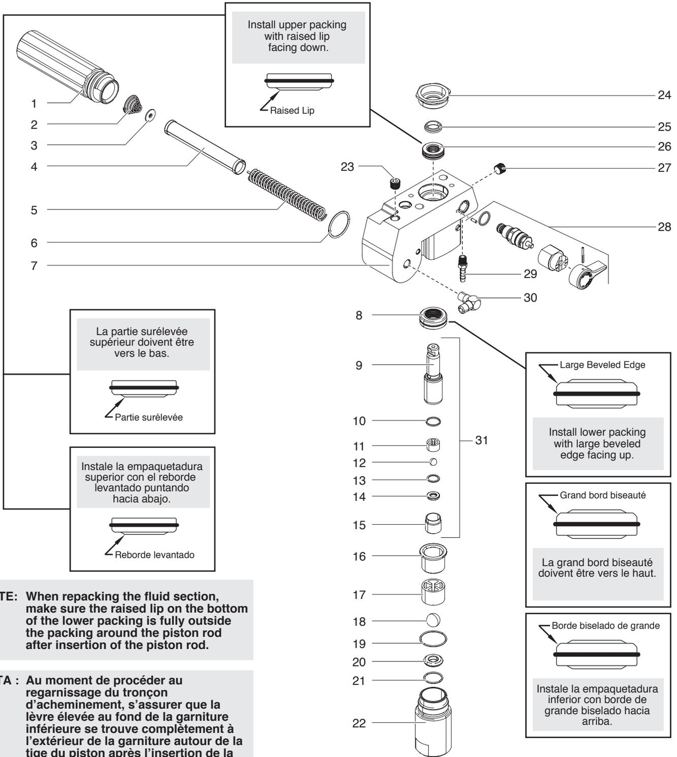
**NOTE:** When repacking the fluid section, make sure the raised lip on the bottom of the lower packing is fully outside the packing around the piston rod after insertion of the piston rod.
