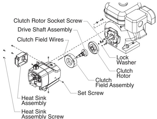
**NOTE: To remove the drive shaft assembly, the pump housing first must be removed from the gear housing.**
