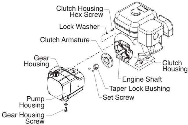
6. Locate the clutch armature assembly on the end of the engine shaft. Note the two set screws as well as the unused, threaded hole in the taper lock bushing at the center of the clutch hub.
