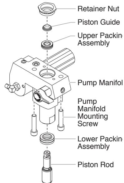
2. Using 3/8" a hex wrench, loosen and remove the two pump block mounting screws.
