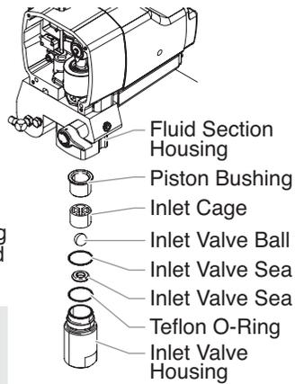
**NOTE: Keep the sprayer in the upright position for this procedure.**
