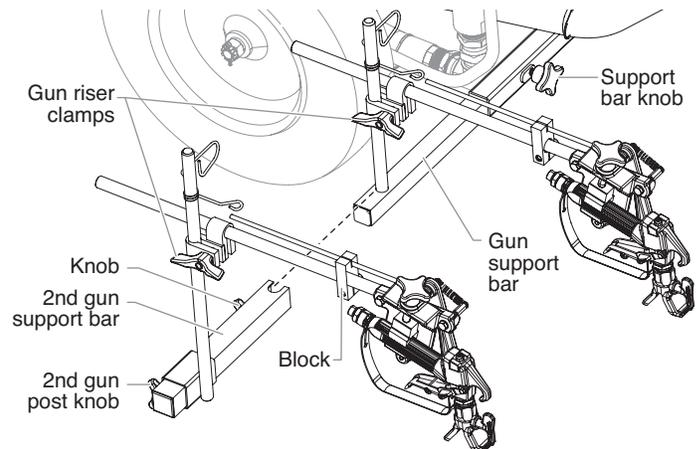
**NOTE: The gun support bar and the spray gun(s) can be mounted on either side of the sprayer. Refer to the "Spray Gun Positions" illustration near the back of this manual.**
