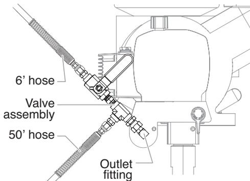
3. Attach an airless spray gun to each of the spray hoses. Using two wrenches (one on the gun and one on the hose), tighten securely.
