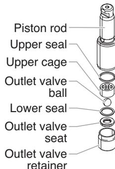
**NOTE: If the outlet valve seat is reversed or replaced, the outlet valve ball must be replaced.**
