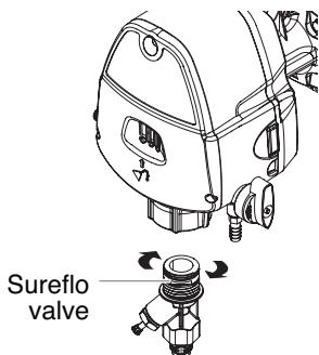
**NOTE: If priming problems continue, you may need to replace the Sureflo valve. Contact Technical Service to order a new Sureflo Valve assembly.**
