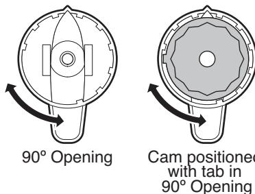
14. Slowly turn the knob counterclockwise until the bottom of the knob moves out to where it is flush with the bottom of the cam (approximately 5-7°).
