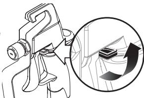
**NOTE:** If necessary, loosen the gun holder clamp knob and then engage the spray gun trigger lock. Move the spray gun to its original position and tighten the clamp knob.
