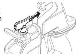
**NOTE:** If the tip is difficult to rotate, relieve pressure by 1) slowly turning the PRIME/SPRAY knob to PRIME, 2) unlock the spray gun, and 3) squeeze the spray lever. Release the lever, lock the spray gun, and try rotating the spray tip again.
