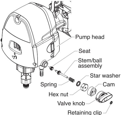
6. Tighten the new stem/ball assembly seat into the pump head. Use a 7/32" hex wrench. Torque to 6-8 ft./lbs.
