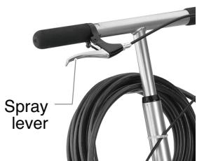
**NOTE:** The sprayer is equipped with an automatic safety shut-off switch to prevent the sprayer from overpressurizing. When the PRIME/SPRAY knob is in the SPRAY position, pulling and holding the spray lever half way without triggering the spray gun will engage the safety shut-off switch. Refer to the Maintenance section if the safety shut-off switch engages.
