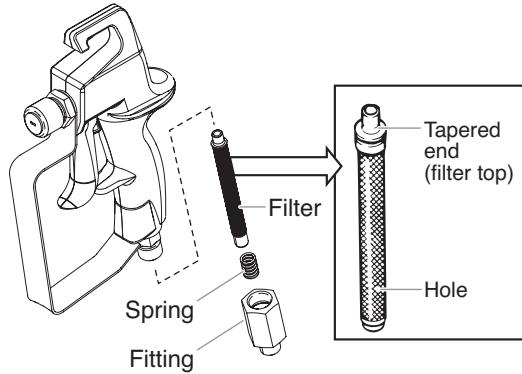
**NOTE: Never poke the filter with a sharp instrument!**
