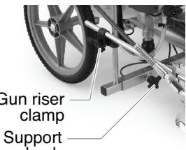
**NOTE:** The height of the spray gun affects the width of the spray pattern (i.e., the lower the gun, the smaller the line width). Tip size also affects line width.
