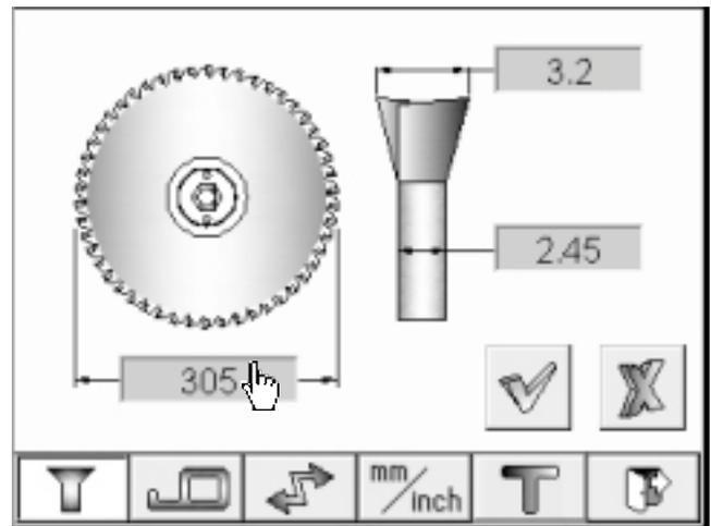
Step 2: Input 14" saw blade's specification, push  key to finish input. For the remaining value, the input way is the same.
