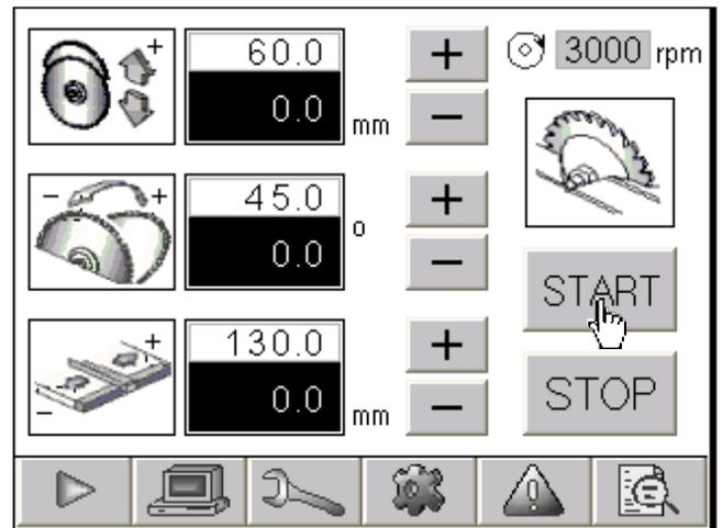
Ex 2: If the total length and the desired cutting size are known and you want to calculate the size of the remaining material, the operating way as follows:
