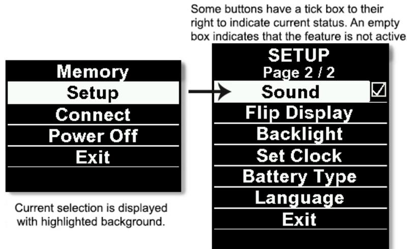
To navigate, use the **Up** and **Down** buttons to scroll vertically and
