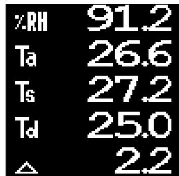
**Advanced models** allow the user to set up custom alarm conditions for each reading in a dataset. Use the **Up** and **Down** buttons to scroll through each value and corresponding operator.
