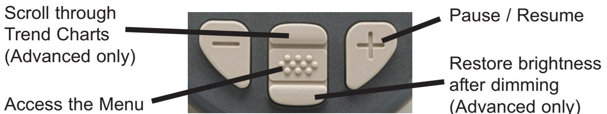
The Pause/Resume (+) button stops values from automatically updating to allow for closer examination of the relationship between the values or to allow time to manually record the entire dataset. Press (+) again to resume.
