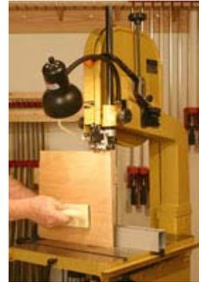
With the addition of our riser block kit, the PWBS-14 resaw capacity increases to 12" from the upper guide to the table surface!
