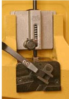
A Carter Quick Release lever (left) is standard on the Powermatic PWBS-14 and makes fully relaxing blade tension quick and easy. The Quick Release lever works independently of the blade tensioning block (right) so the setting is not lost between uses.
