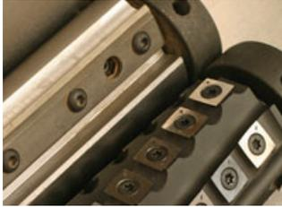
The helix head (right side of the image) uses full carbide inserts that greatly extend durability as well as the quality of the cut. Sound is also drastically reduced over nearly all other cutter configurations.
