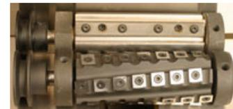
The 54A cutterhead (top in this photo) features our Quick Set knife system that uses cams to position the knives precisely so they cut smoothly and work together equally to disperse wear.
