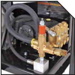
Belt drive triplex piston General pump with ceramic plungers
