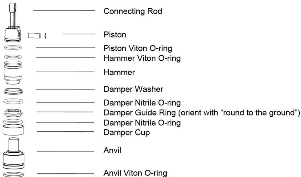
**Figure 9: View of the orientation of internal parts**
