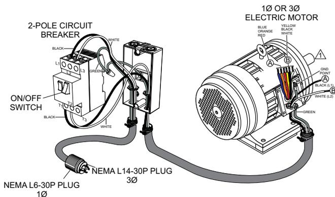
Figure 5. Electric Motor
