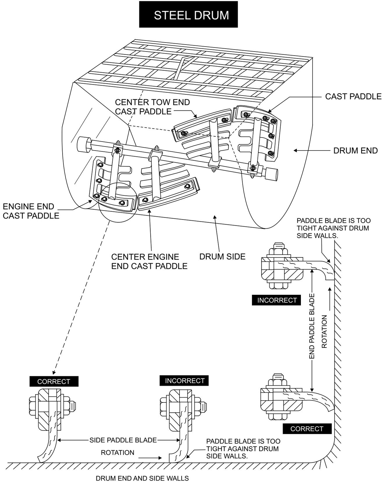
Figure 6. Paddle Blade Adjustment
