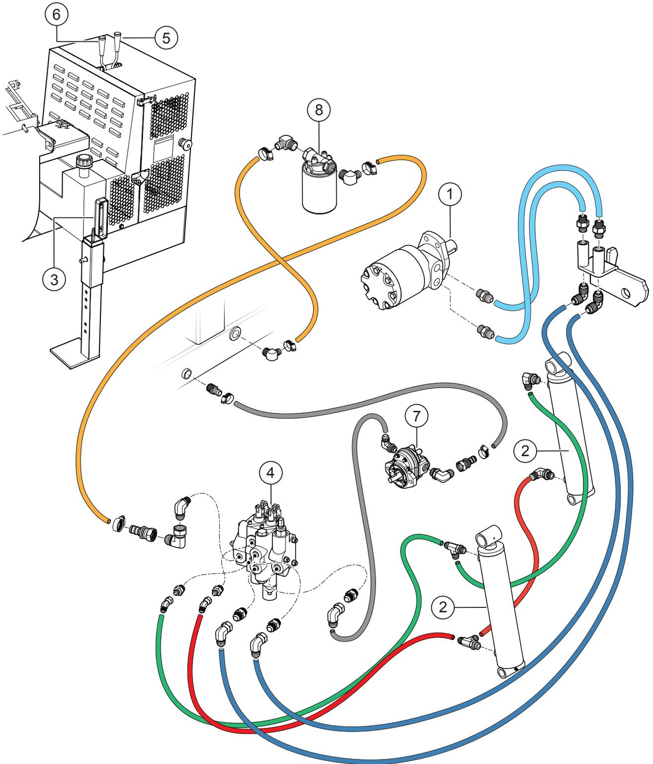
Figure 3. Hydraulic Components
