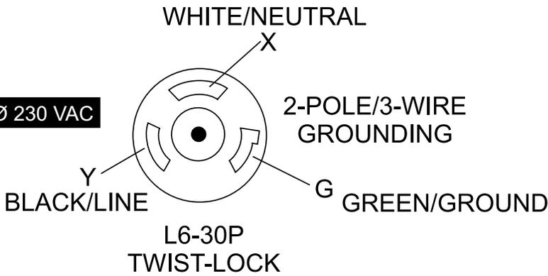
230 VAC WINDING CONNECTIONS (LOW VOLTAGE)
