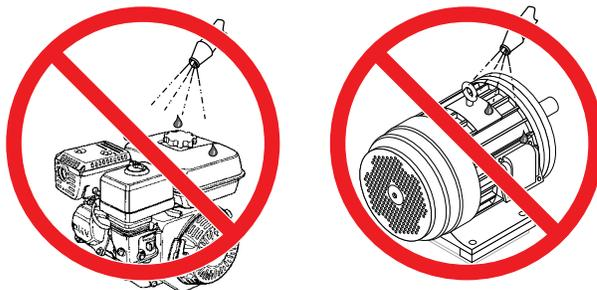
Figure 33. No Spraying of Water
