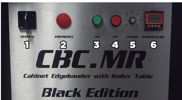
1. Turn the main switch (1). This key energizes the machine's panel, without turning it on.
