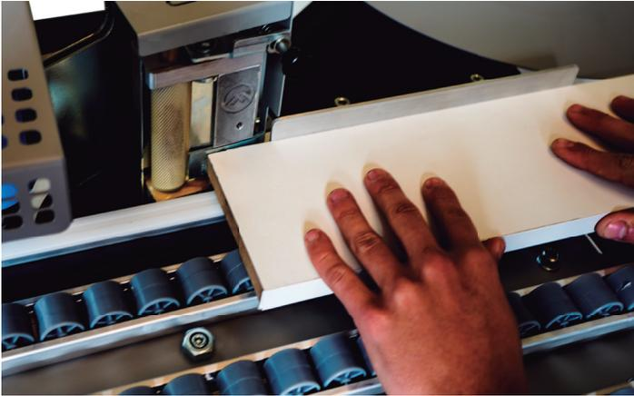
**CAUTION.** Crushing and cutting risk. Do not bring your hands within 10cm (4") manual cutter. Do not wear loose clothing or gloves when operating this equipment.
