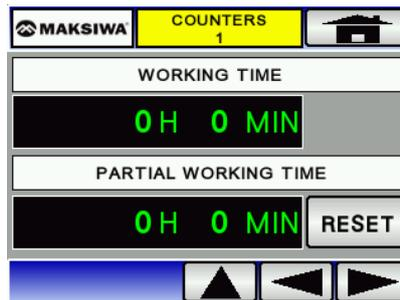
**WORKING TIME** – Total hours machine working time.
