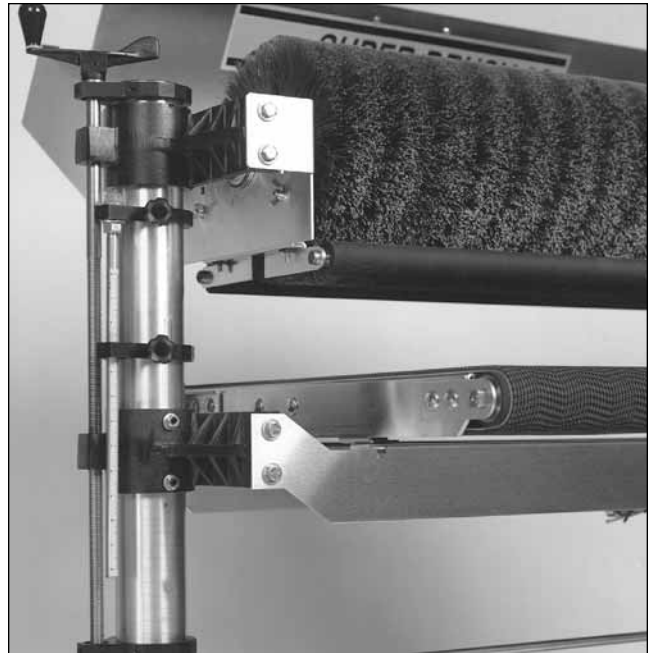
Fig. 6. Checking brush alignment and table height adjustment (outboard side).
