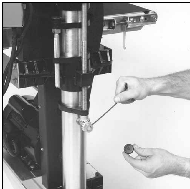
Fig. 14. Adjusting miter gears for proper mesh.
