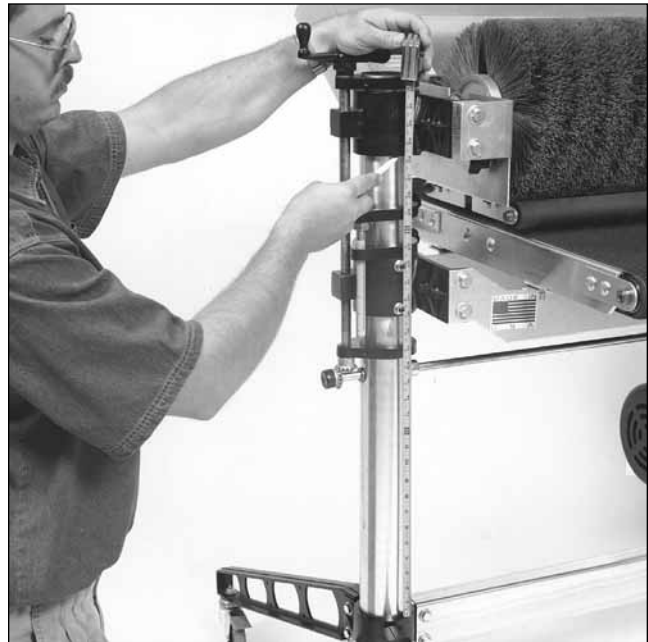
Fig. 18. Comparing brush support casting heights.
