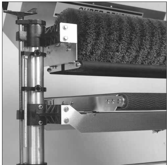
Fig. 16. Height controls on outboard side.
