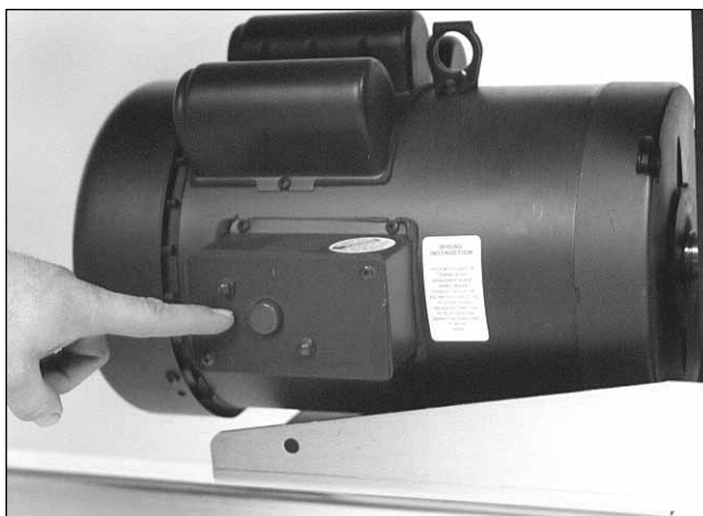
Fig. 4. Thermal-overload switch, on some models.
