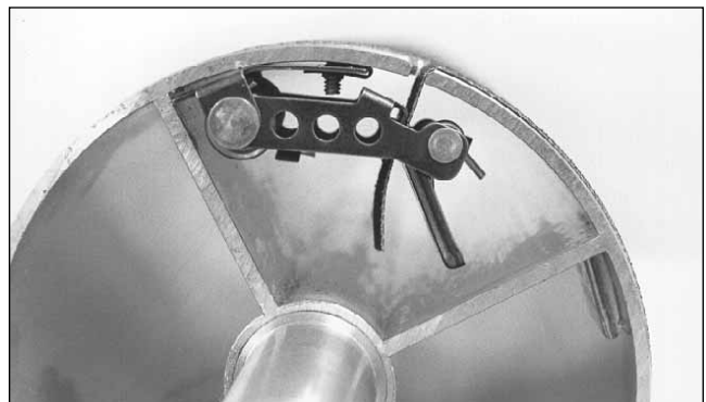
Fig. 12-i. Reset take-up as needed as strip stretches.
