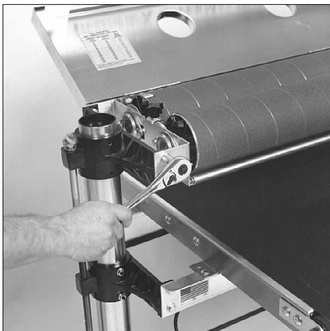
Fig. 31. Drum support casting bolts (outboard side).
