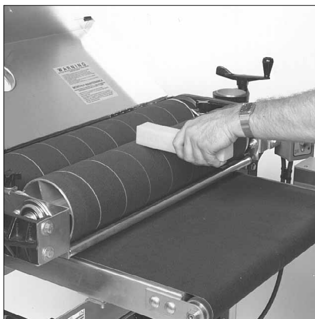
Fig. 18. Cleaning abrasive strips.
