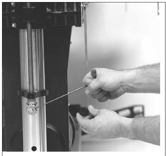
Fig. 7. Checking drum alignment (inboard side).
