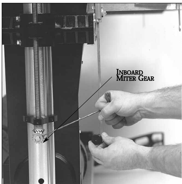
Fig. 8. Adjusting primary drum alignment.
