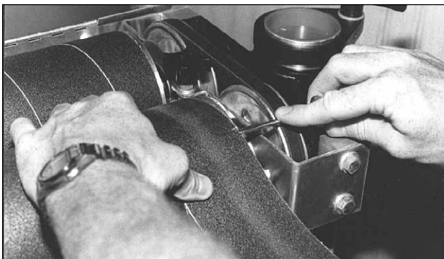
Fig. 12-f. Mark strip where it crosses drum edge.
