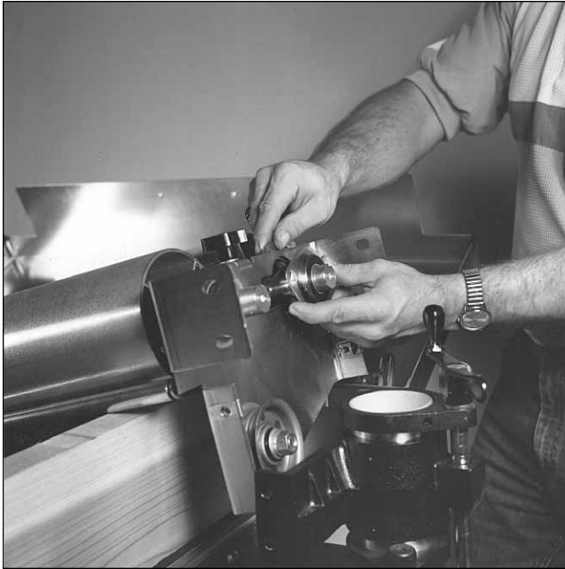
Fig. 43. Removing rear bearing (inboard side).
