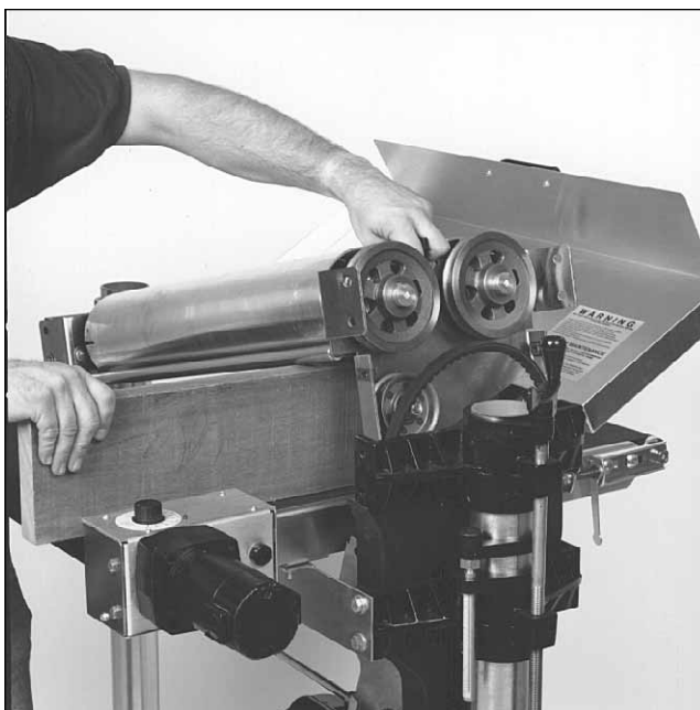
Fig. 32. Supporting drums with 2x6 on edge.
