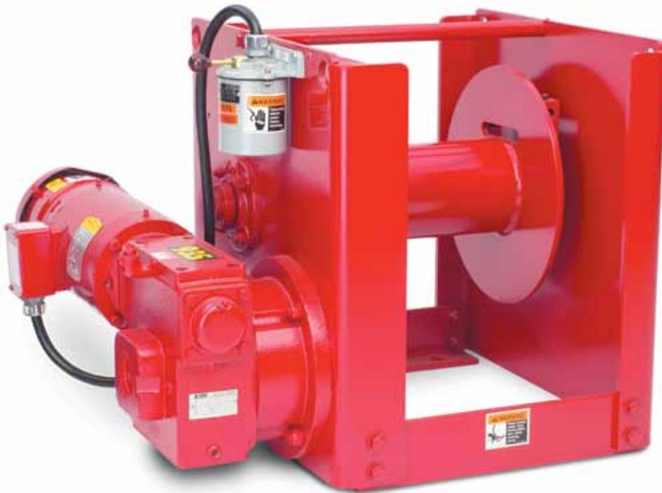
**FLANGE MOUNTED MOTOR** is a 230/460 volt 3 phase motor, 60 cycle, IP 54<sup>1</sup>, TEFC severe duty, reversible, class B or F insulated, continuous duty brakemotor.
