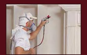
The ADVANTAGE 400 was designed to minimize size and weight without sacrificing performance. We built this unit to deliver .47 GPM — making it the highest performing sprayer in its class and therefore ideal for smaller residential and commercial applications.
