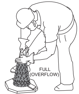
Figure 55-C. Slump Test (Full-Overflow)
