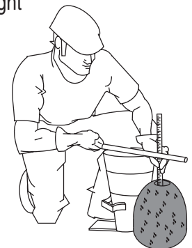
Figure 55-F. Slump Test (Measurement)
