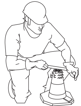
Figure 55-D. Slump Test (Removing Excess Concrete)
