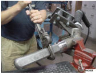
Secure vibrator bracket in vice and allow the bracket gusset to work as a stop against the vice jaws. Unscrew the head assembly from the vibrator bracket.
