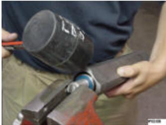
If the rotor assembly does not freely fall out of the head housing, clamp the flat sides of the driver sleeve in a vise. Pull the head housing off of the rotor assembly using a soft tool so no thread damage will occur.
