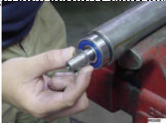
Clamp the rib of the rotor in a vise. Unscrew the driver sleeve (left hand thread). Remove the spacer from the rotor. Unscrew the hex nut from the opposite end of the rotor (left hand thread). Remove washer, the remaining two
