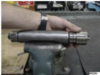
Slide the bearing cup evenly across the bearings at the driver. Grease the smaller driver to the drive sleeve.
