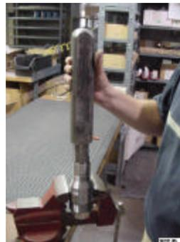
Slide the housing over the bearings until it reaches the threads. Apply Permatex to threads and continue to turn until it is fully tightened.
